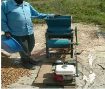
Figure 23: A ground nuts thresher at home is a good value addition and labour-saving equipment
